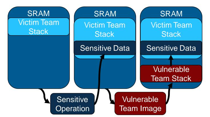
By leveraging these leaks, we successfully extracted private keys and pairing pins on the test boards. However, this **attack did not work on keyed boards** since the bootloader clears the SRAM and removes any sensitive data left by the victim team.
