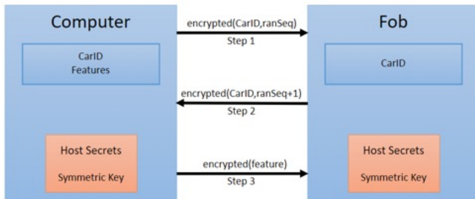
Figure 2: Initial Process to Enable Feature on a Paired FOB
